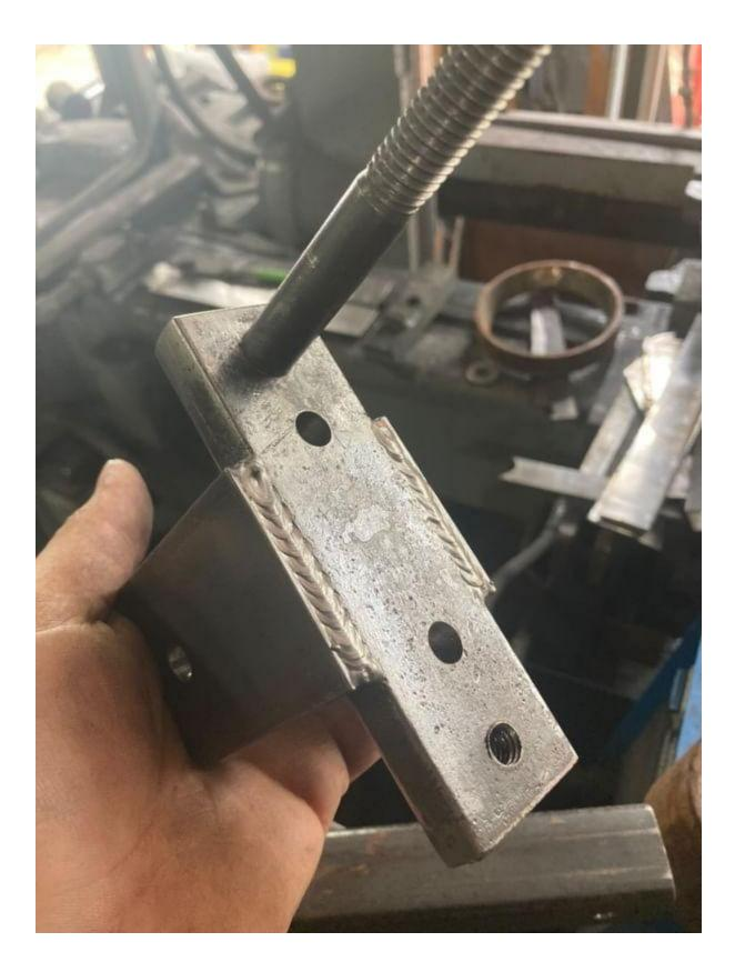
Pivot assembly detail. 1/2" threaded shaft plug welded in one end, 3/8" threaded hole in other end for adjustment screw. Pivot ears welded to tracking plate. Remove the paper shim for a nice fit.
