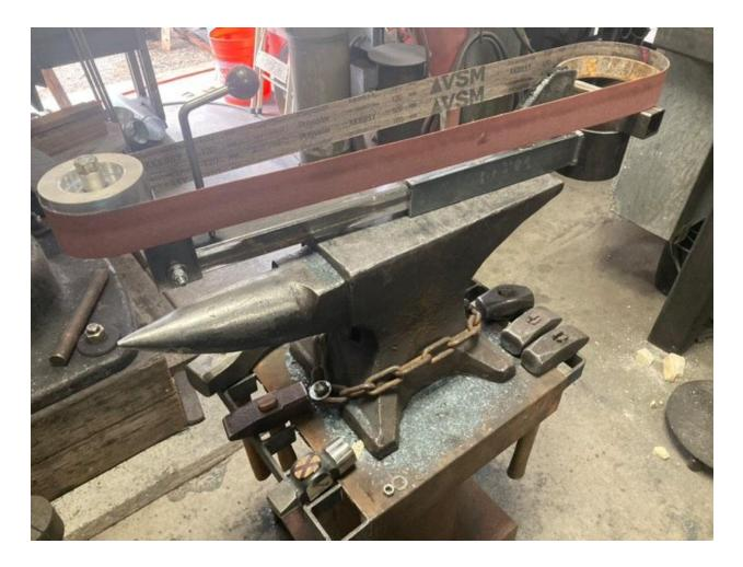
Once the idler arm is trimmed to length weld cap to end to push on the spring. Spring can also be shortened if need be. Another option is to add shims inside of the receiver arm to adjust tension.
