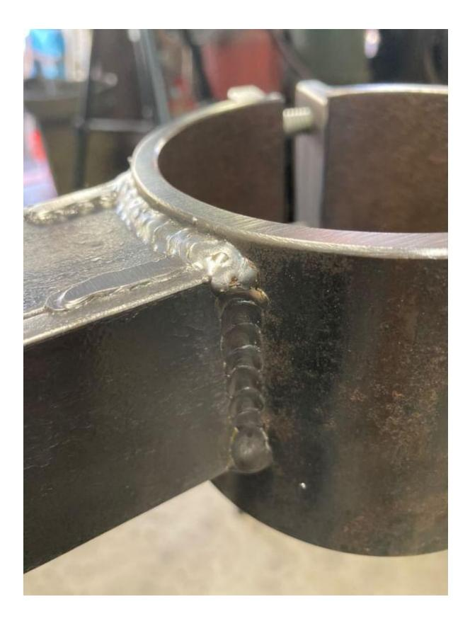
Top of idler arm tracking assembly. Match drill for pivot bolt, drill pivot hole in arm top, bolt ears to frame with paper shim on one side. Ears are chamfered for weld on top as shown.
