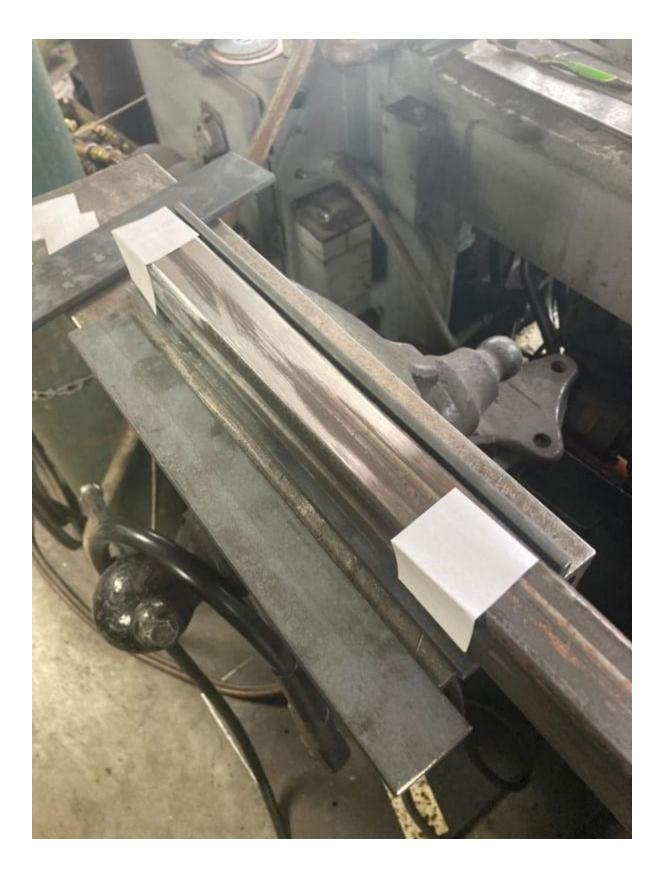
The welds on the receiver do not need to be large (about 1" is enough) as it is a guide component and warpage would be detrimental to the fitment. Remove the arm while still hot and lightly grind on the sides if need be until it slides freely.
